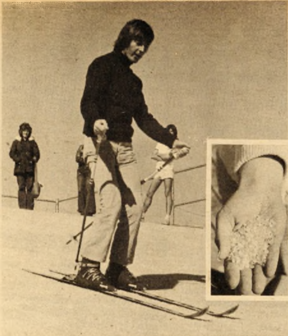
The synthetic slope shown here is made of loosely-spread plastic granules (see photo insert).
