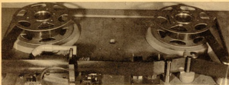
SPEED DEMON —This "gadget," part of Foothill's Video-tape recorder, is the secret of the machine's success. Inside of the "video head assembly" on the lower left, four little heads spin at 90 MPH at right angles to the tape.
