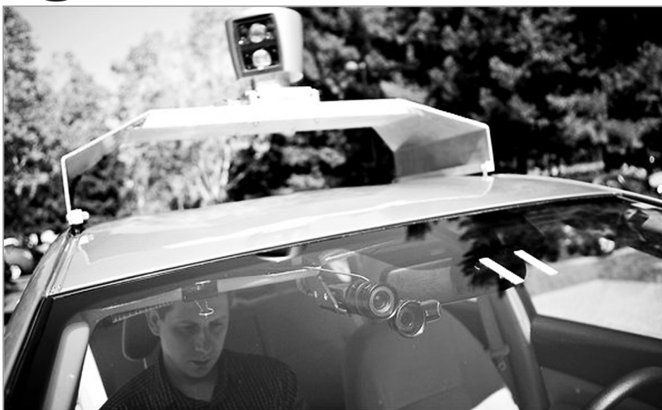
SENSORED DRIVING - Google's driverless car uses cameras to judge distances from other objects.
