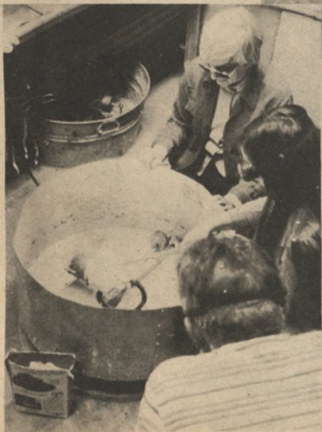
Joyce Hendry, instructor, gives advice on melting metal for a cast in the centrifugal casting machine.
