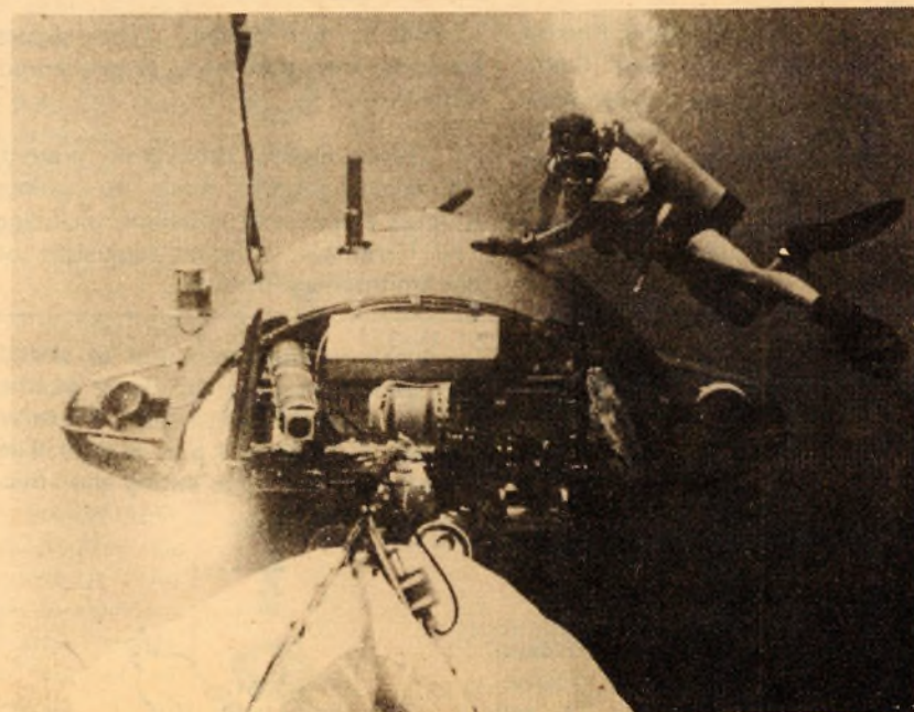
EXPLORING THE OCEAN DEPTHS. Diver checks a net for collecting specimens that is attached to Westinghouse Deepstar 4000, a deep diving submarine research vessel.
